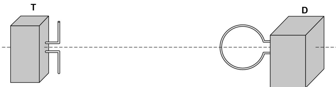
**T** is a radio wave transmitter with an aerial consisting of two vertical metal rods.
