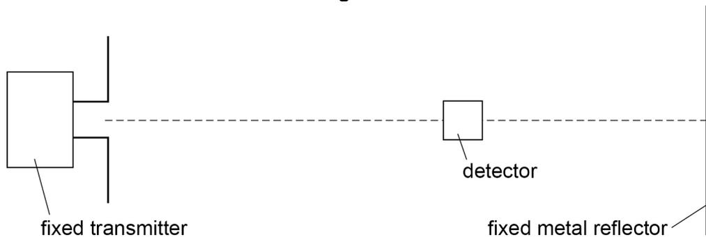
Stationary waves are produced between the fixed transmitter and the fixed metal reflector.
